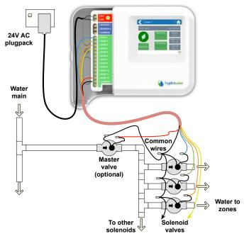
1. Take one wire from each solenoid, twist together and connect to the common (usually black) wire of your multi-core irrigation cable.
