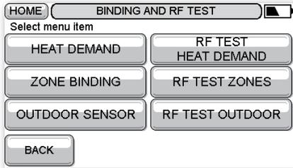
**Binding** will normally be performed with evotouch positioned beside the actuator or sensor, for convenience.
